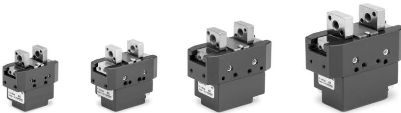
Series CGSP grippers, available in 4 sizes (20, 25, 32 and 40) are parallel and double acting, self-centering and guided by means of a T-shaped sliding guide. Thanks to the materials and surface coating used, the gripper offers a high reliability. Moreover, the internal force transmission system is protected against the entrance of impurities by means of a steel cover so the gripper can also be used in dusty environments.
