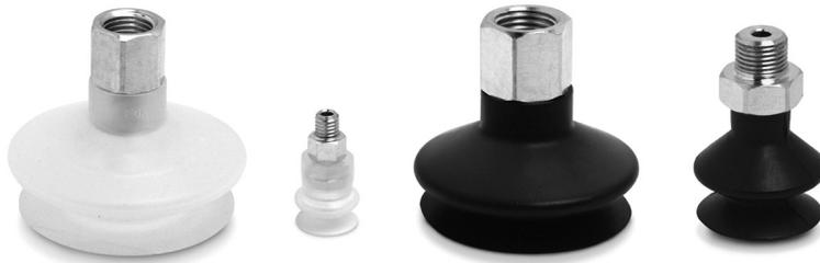
Series VTCL bellows suction pads (1,5 folds) have a rugged design and consist of a nipple and rubber part. The nipples are inserted directly into the rubber part. The rubber parts can also be ordered separately without nipples as spare parts. Materials: NBR or Silicone
