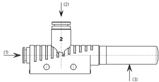
Usable fluids: compressed air, oiled and not, according to ISO 8573-1:2001 class 7-4-4
