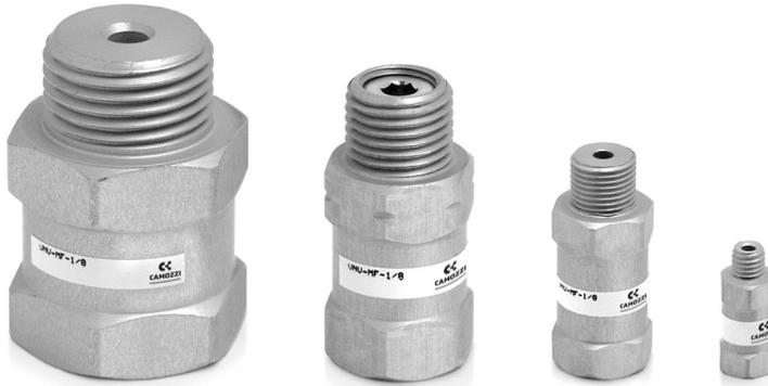
The check valves Series VNV are mainly used on vacuum gripper systems containing multiple suction pads in order to shut off individual suction pads which are not covered or accidentally pulled away from the workpiece. In this way the gripper system can operate correctly maintaining the vacuum level necessary for the application.
