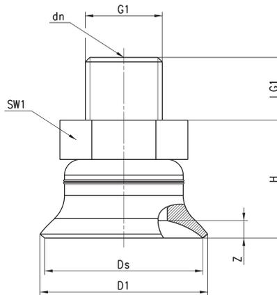
Tolerances for elastomer parts according to M3 - DIN 7715
