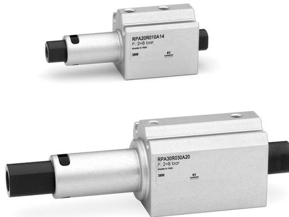
The Series RPA short stroke cylinders are double acting actuators with aluminium hollow through rod and mounting stud. Available in two sizes,  $\varnothing$  20 and  $\varnothing$  30 mm, with different strokes and dimensions of the mounting stud, these actuators are equipped with the non-rotating function of the rod.
