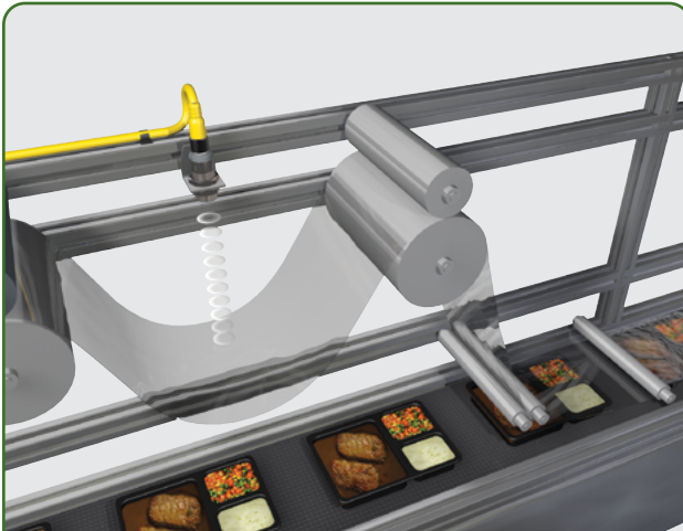
Film position detection - An 873M ultrasonic checks for continual feed of a clear wrap while monitoring tension.
